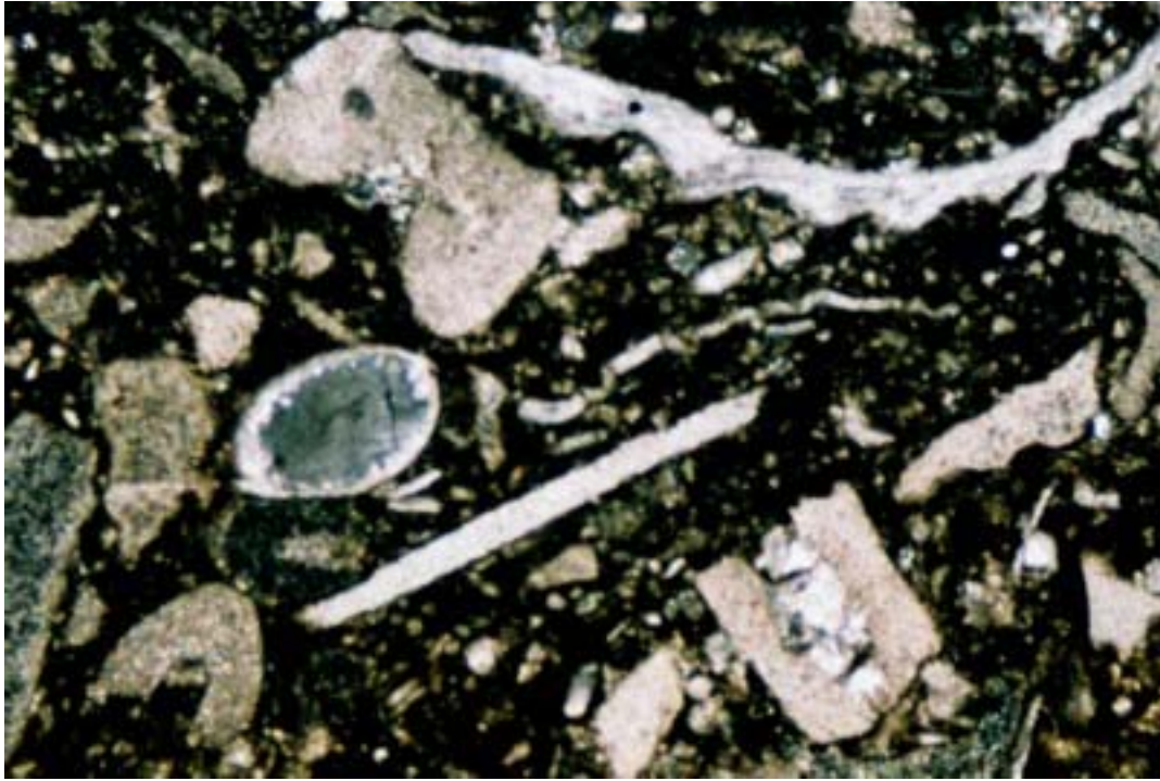
A. Large, partly recrystallized fossil fragments in dark, lime mud. X-axis of photo: 2.3mm. XN.
