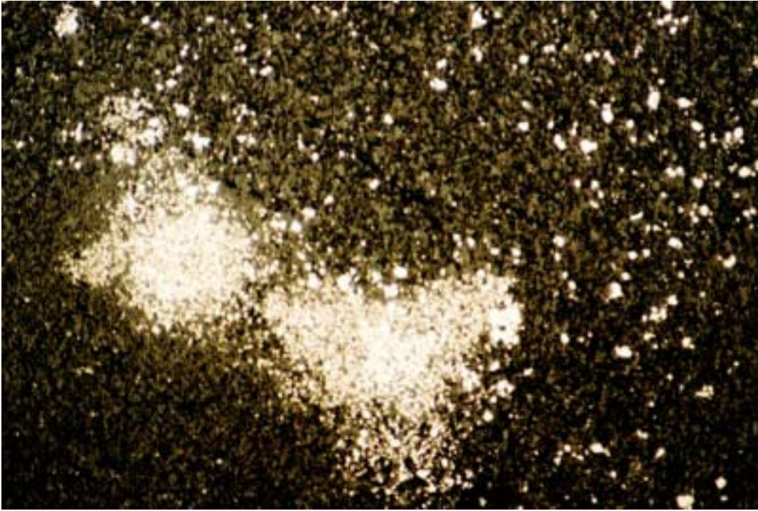
A. Fine-grained aggregates and single grains of pyrite in mudstone. X-axis of photo: 2.3mm. Refl. Light.
